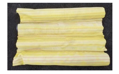
4. On both sides of the mat, 2 inches from the open ends, sew two strips of fire hose perpendicular to the firehose on the mat. Sew this piece of firehose to the mat on one side to create a sleeve for hanging or to slide rope through to attach buoys. We used 12 in long hose that is 2 inches wide.
