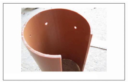
The pipe has a thickness of approximately 5mm. The PVC-U is easy to saw, drill, chamfer and sand (it is not particularly brittle), but is also easily scratched.
